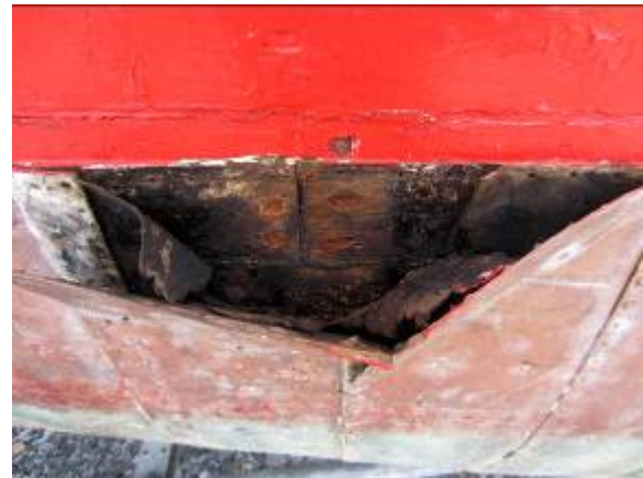
Left: the deck seen from the cargo. Right: planks under the ice sheathing above the waterline.
