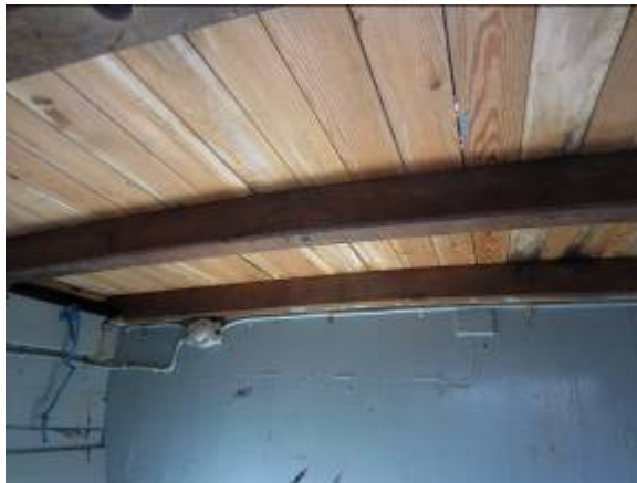
Left: the deck seen from the cargo. Right: planks under the ice sheathing above the waterline.
