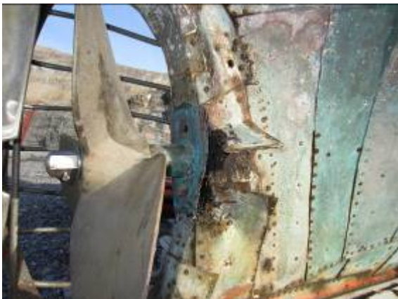
Left: Aft stern is examined. Right: Ice sheathing lifted at for stern.
